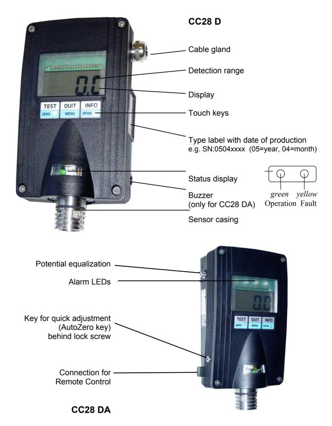
The type label shows the transmitter type. The sensor enclosure includes the sensor and the sensor card, which carries the components for the sensor circuitry. For adjustment of electrical zeropoint and sensitivity you can use either the built-in display or the remote control RC2. A secured key at the left side of the transmitter allows a quick zero setting. The electronics on the main p.c.board converts the sensor signal into a linear output signal of 4 .. 20 mA.
